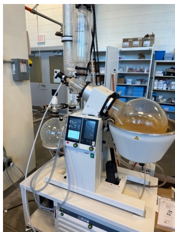
BUCHI Rotavapor R-300 Rotary Evaporator with Controller (3-liter capacity)
