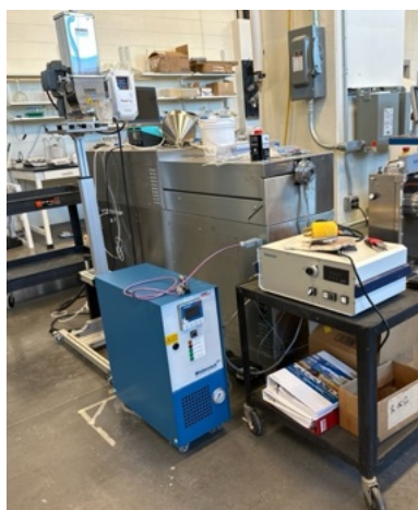
TwinLab-F 20/40 Bradender Extruder (1 - 20 kg/hour)
