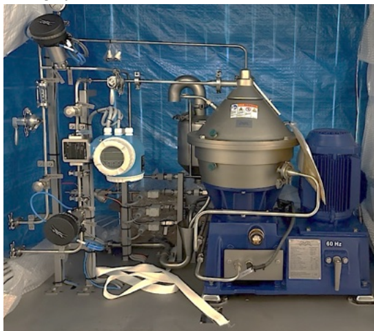
Alfa Laval Clara 20 Clarifier Disk Centrifuge (1,000-liter/hour)
